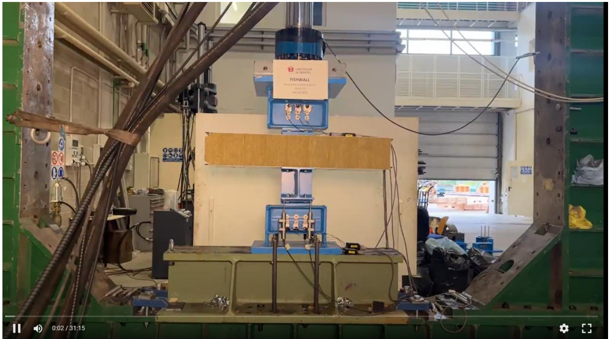
Figure A35. Detail 3.2 - compression test – beginning of the test.
