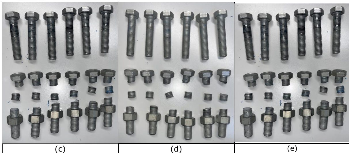
Figure 123. Detail 3.2 aluminium bolts at failure: (a) tension test; (b) compression test; (c) cyclic test 1; (d) cyclic test 2; (e) cyclic test 3.
