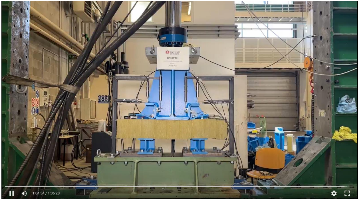
Figure A19. Detail 2 - compression test – deformation at 1 hour.
