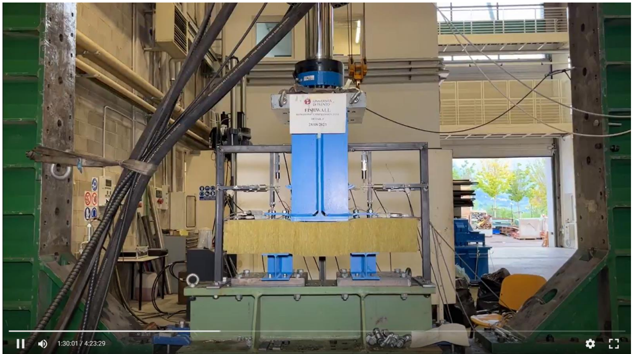
Figure A4. Detail 1 - compression test - deformation at 1.30 hour
