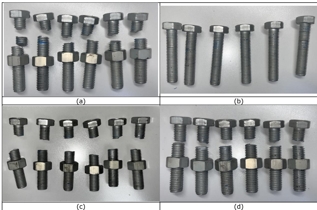
Figure 30. Detail 1 aluminium bolts at failure: (a) tension test; (b) compression test; (c) cyclic test 1; (d) cyclic test 2.
