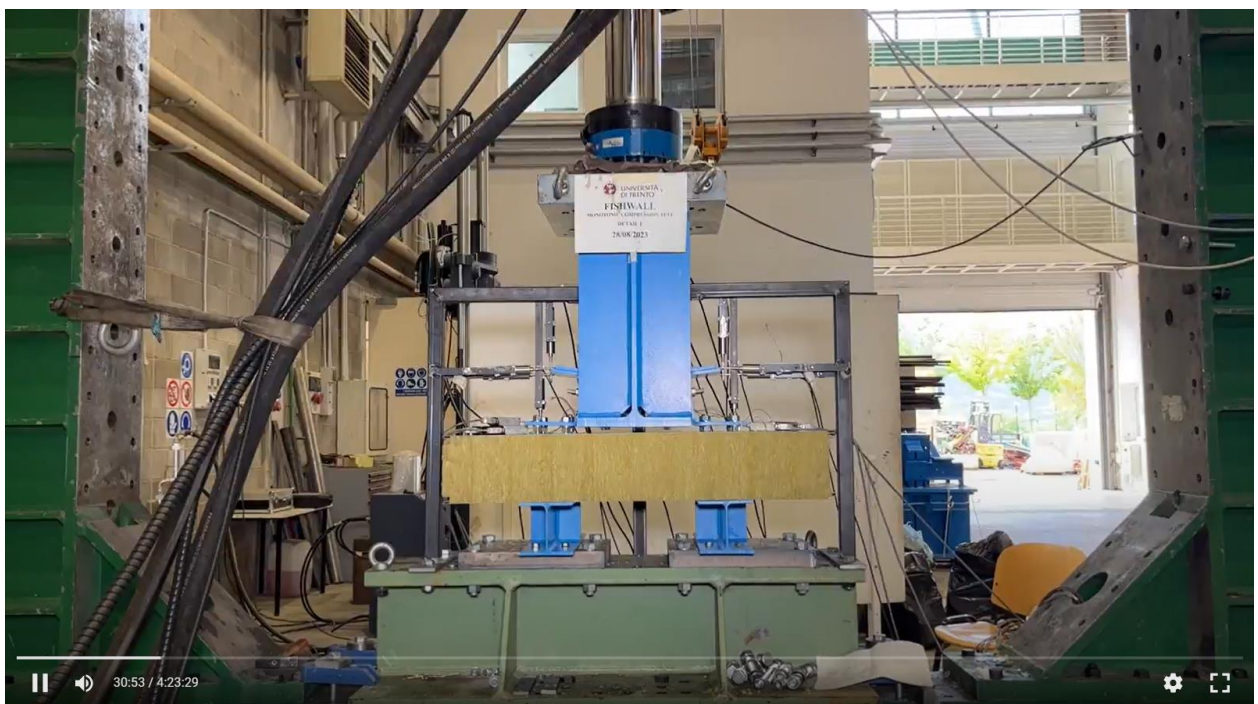
Figure A2. Detail 1 – compression test – deformation at 30 minutes.
