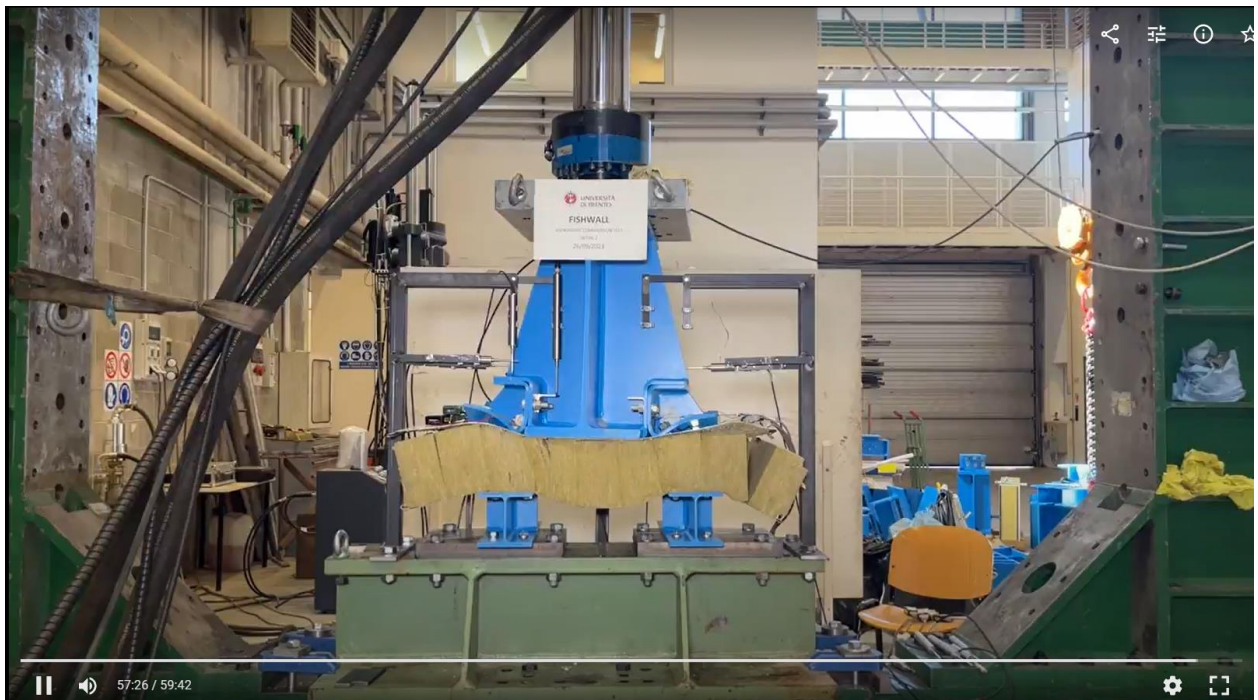
Figure A22. Detail 2 - compression test – deformation at failure.
