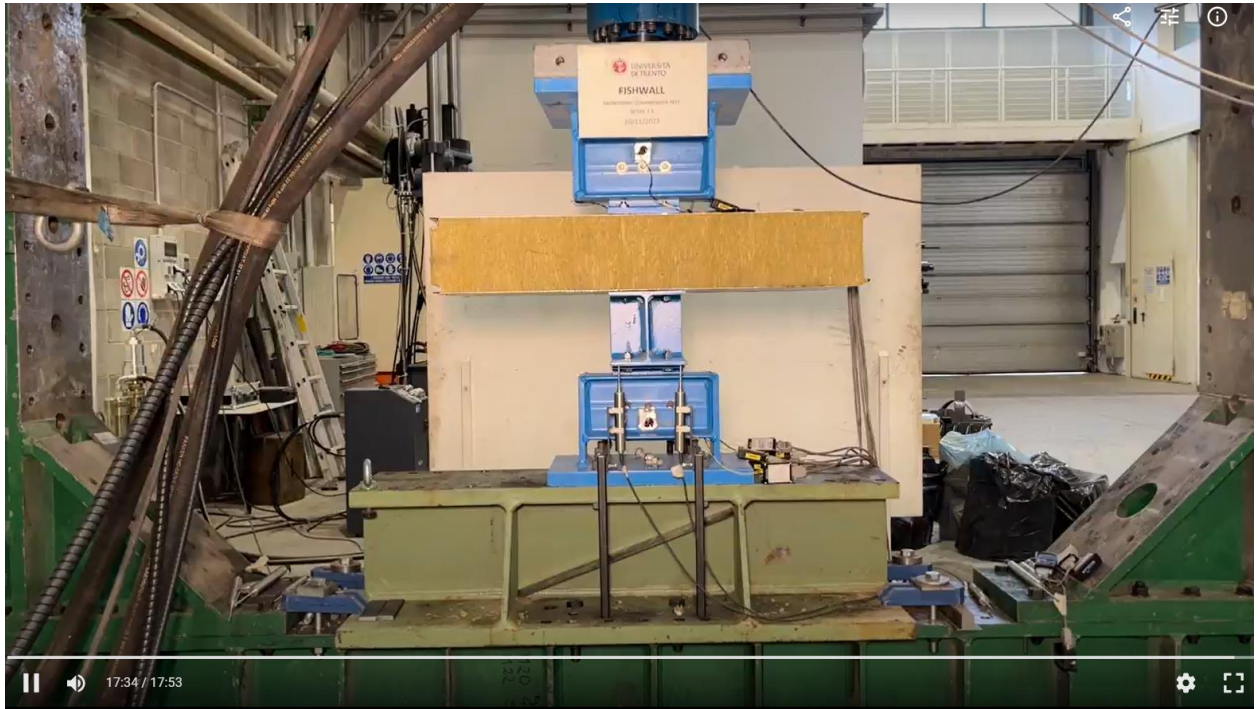
Figure A31. Detail 3.1 - compression test – deformation at failure.
