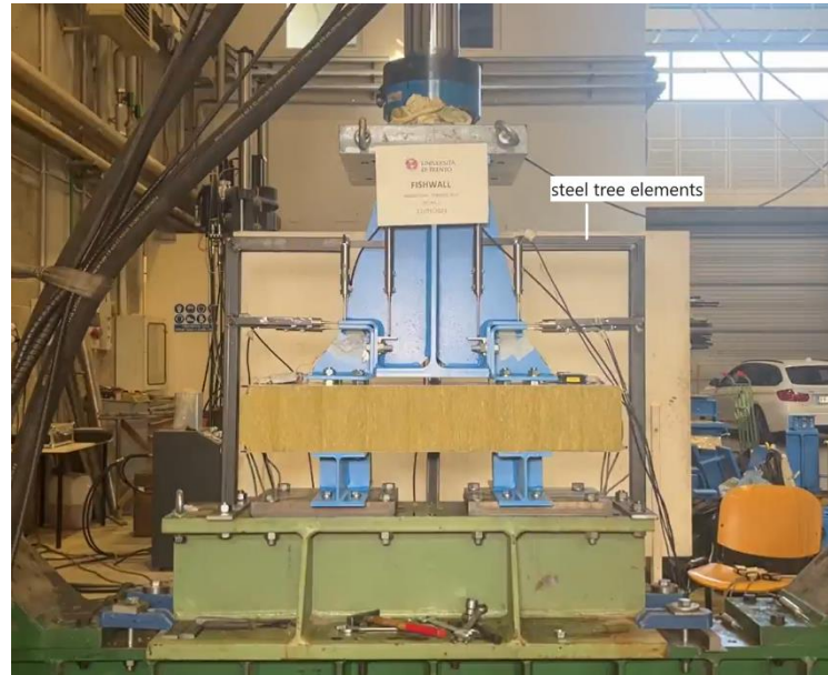
Figure 33. View of the detail 2 test set-up
