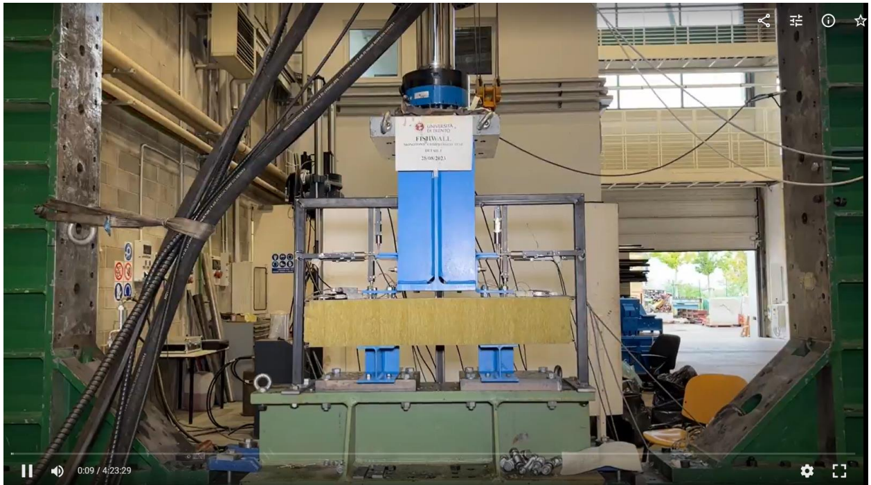
Figure A1. Detail 1 - compression test – beginning of the test.
