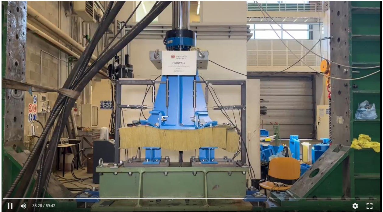
Figure A21. Detail 2 - compression test - deformation at 1.40 hour.
