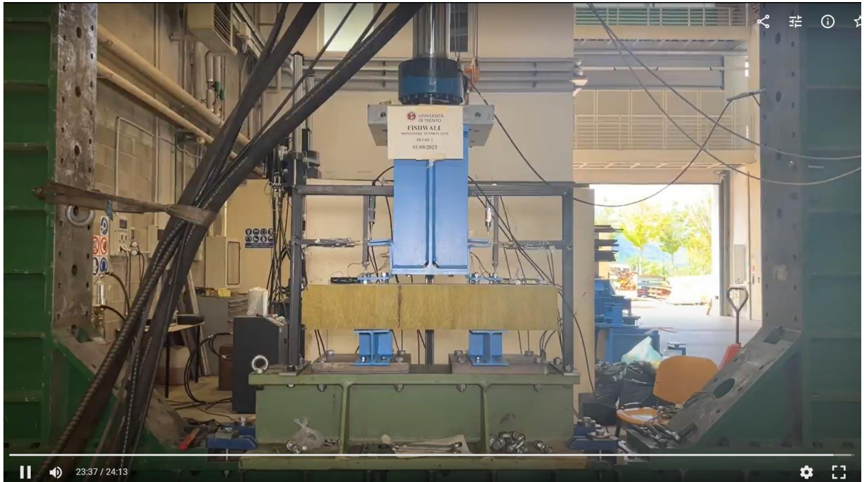
Figure A13. Detail 1 - tension test – deformation at failure.
