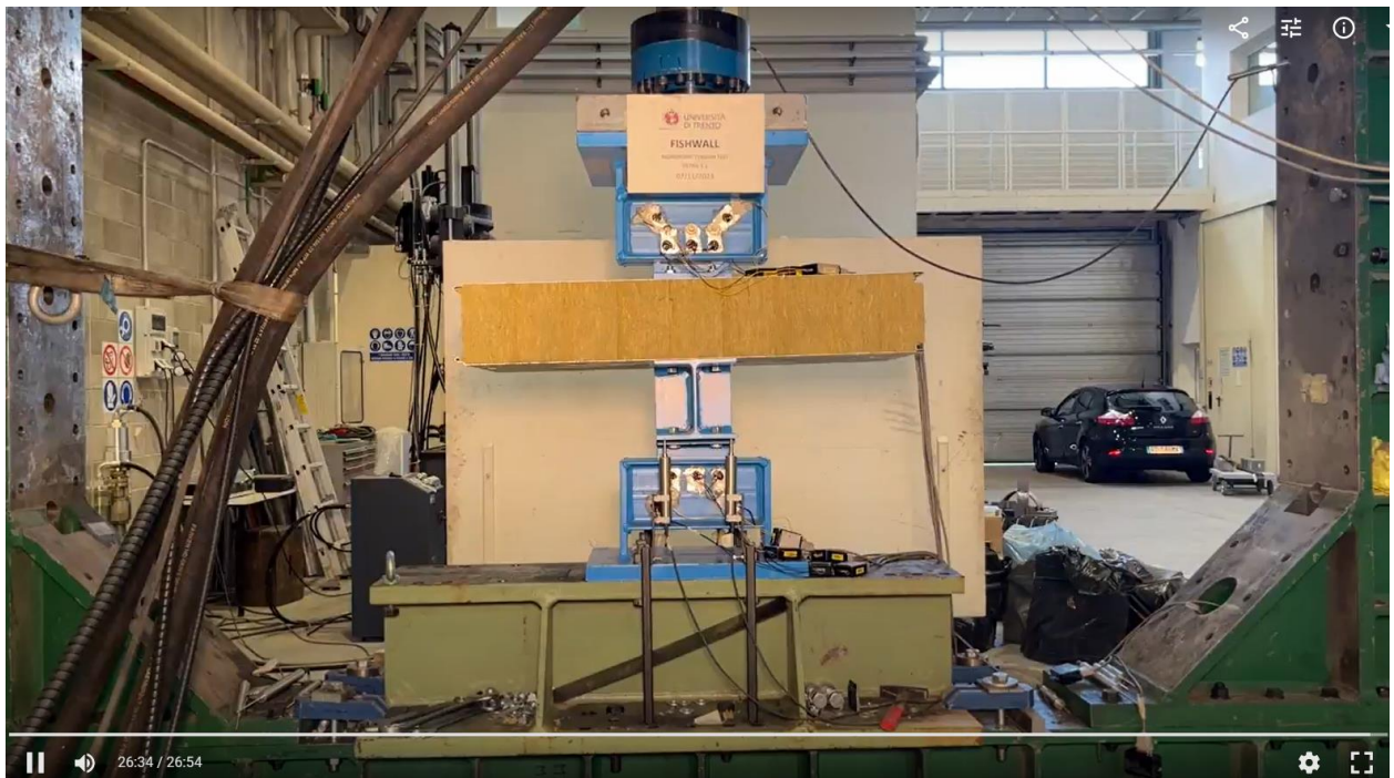
Figure A34. Detail 3.1 - tension test – deformation at failure.
