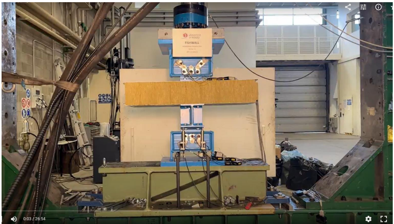
Figure A32. Detail 3.1 - tension test – beginning of the test.
