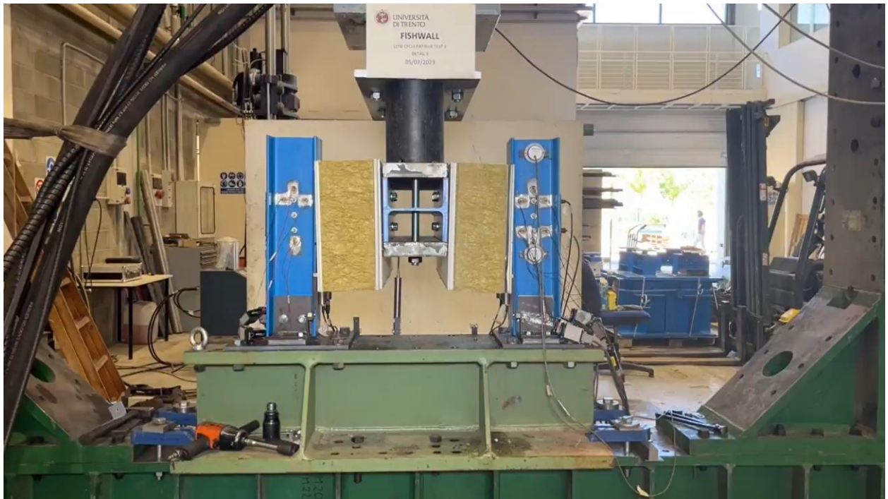
Figure A61. Detail 4 - cyclic test – deformation at +e_y/3
