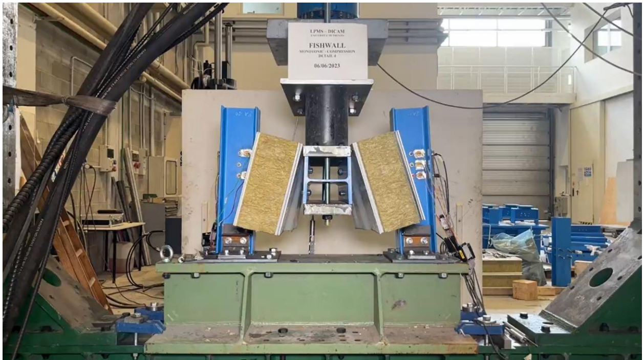
Figure A48. Detail 4 - compression test - deformation at 2.30 hours
