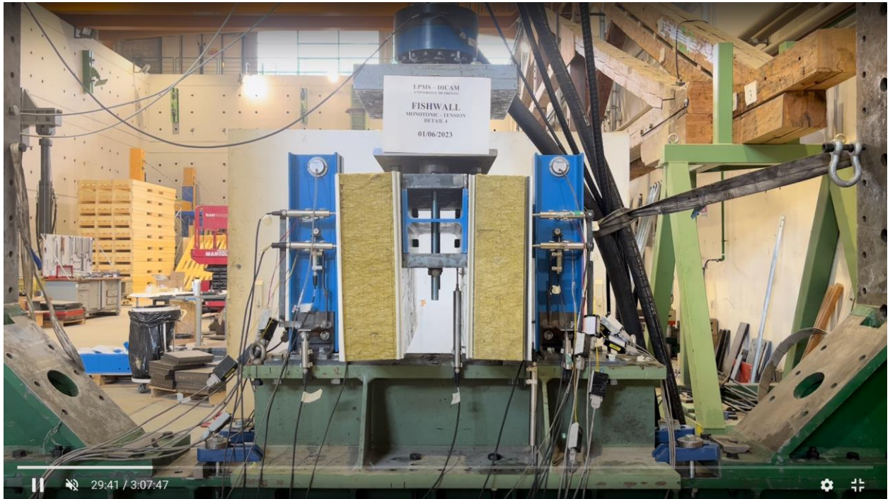
Figure A51. Detail 4 - tension test – deformation at 30 minutes.
