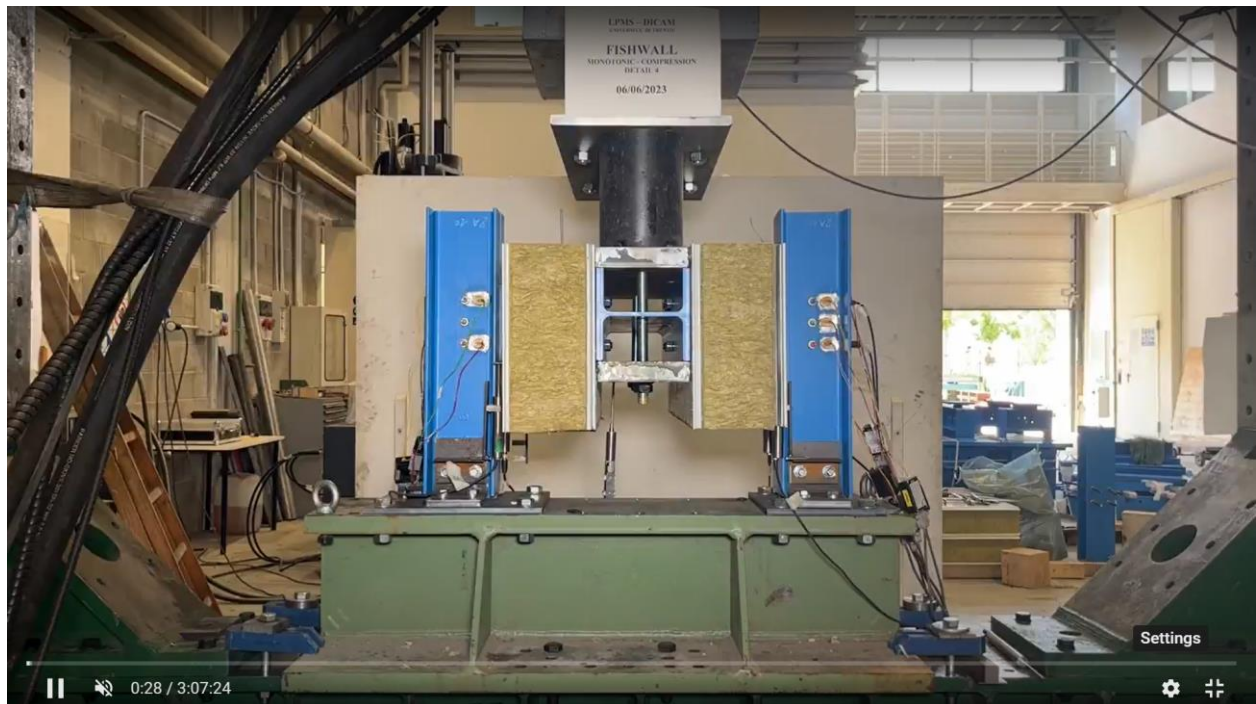
Figure A43. Detail 4 - compression test – beginning of the test.
