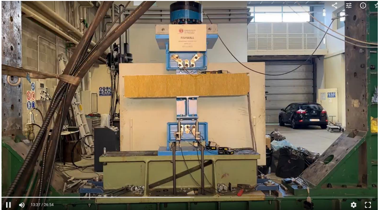
Figure A33. Detail 3.1 - tension test – deformation at 13 minutes.
