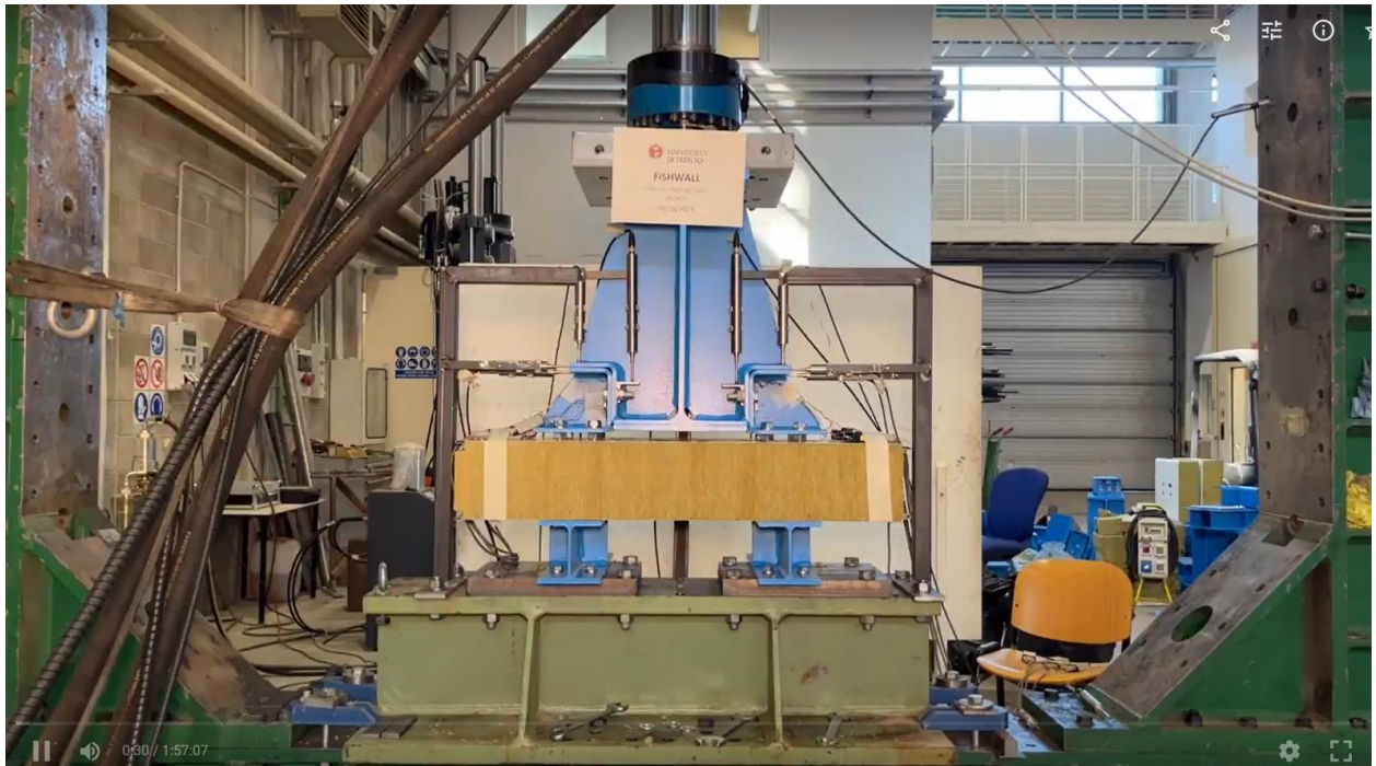
Figure A27. Detail 2 – cyclic test – beginning of the test.
