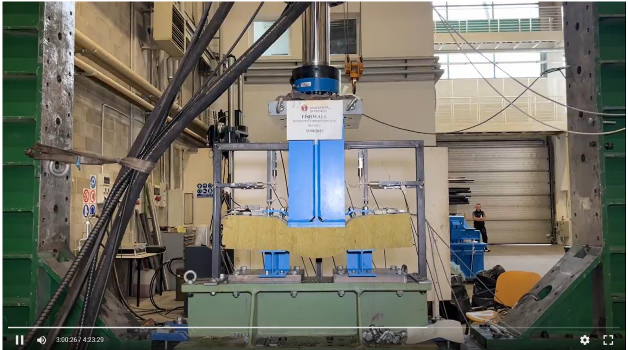
Figure A7. Detail 1 - compression test - deformation at 3 hours.
