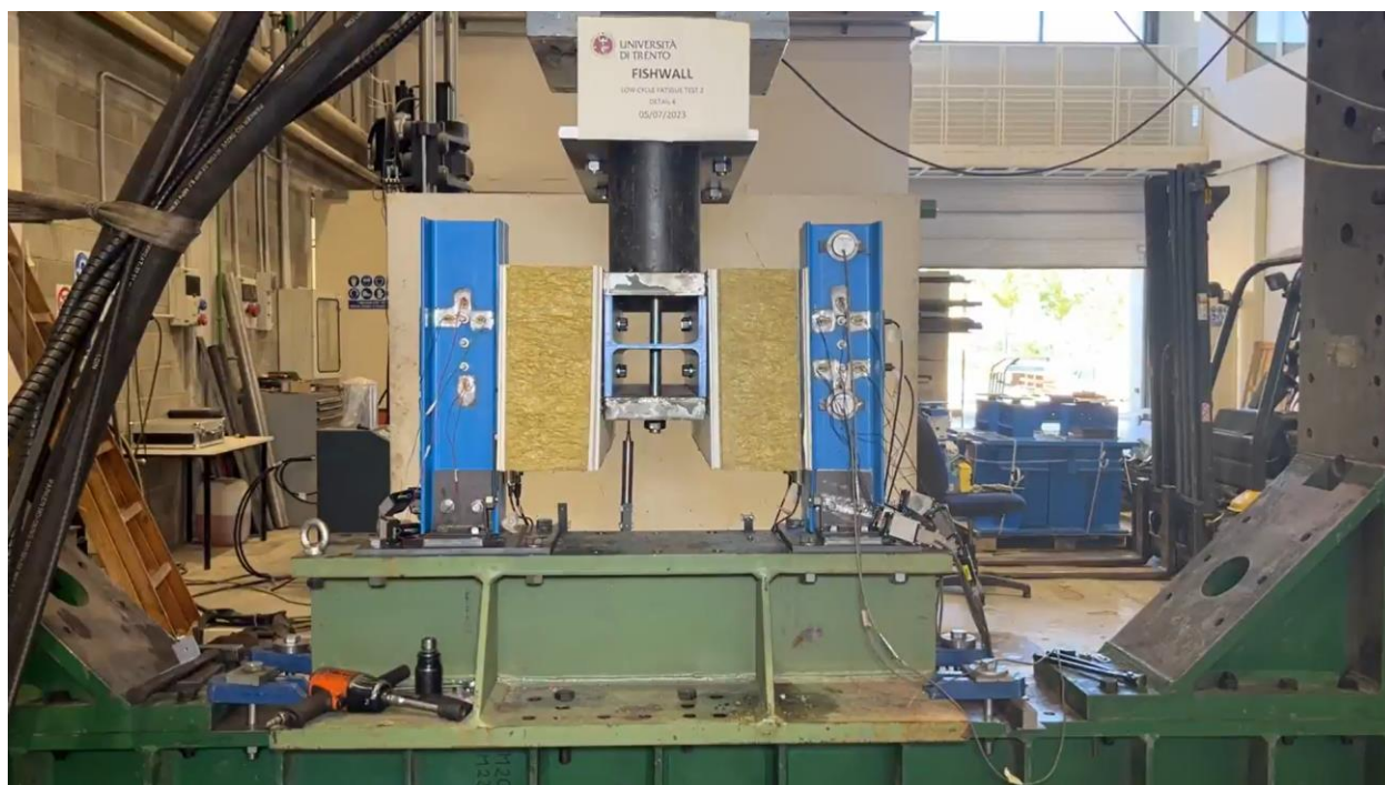
Figure A60. Detail 4 - cyclic test – deformation at -e_y/4
