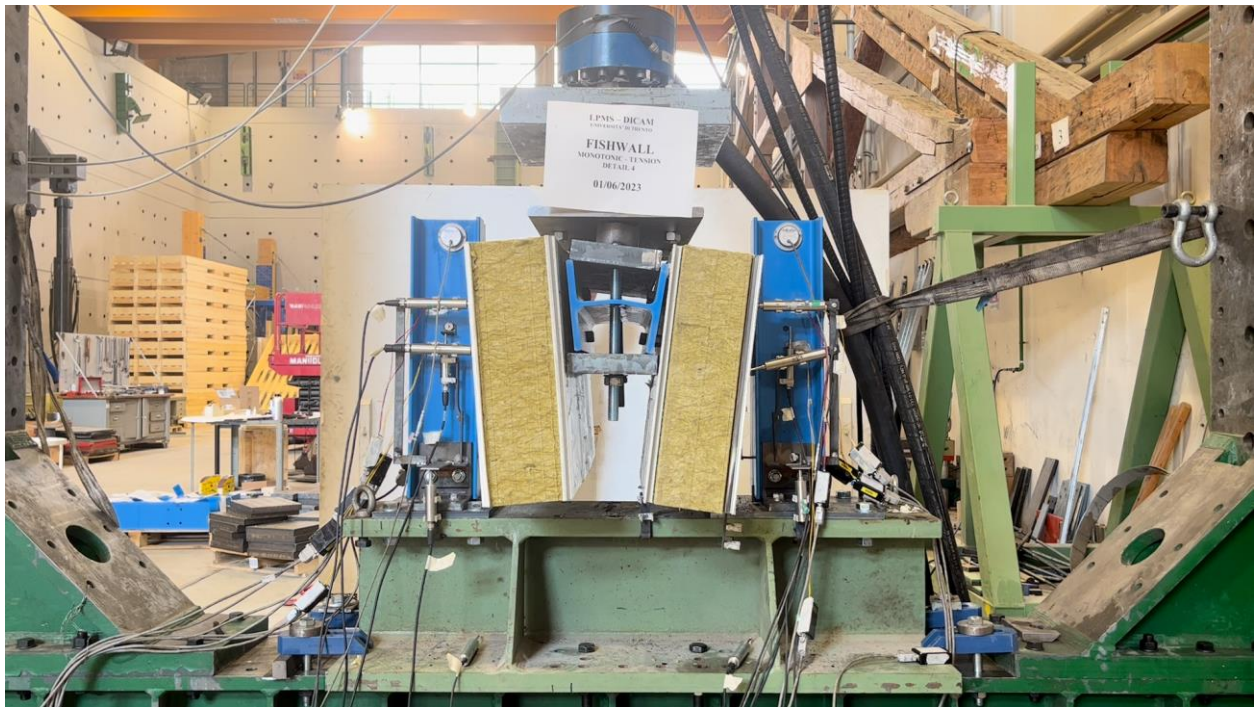
Figure A57. Detail 4 - tension test – deformation at failure.
