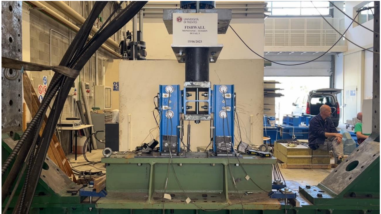
Figure A75. Detail 5 - tension test – deformation at 20 minutes.
