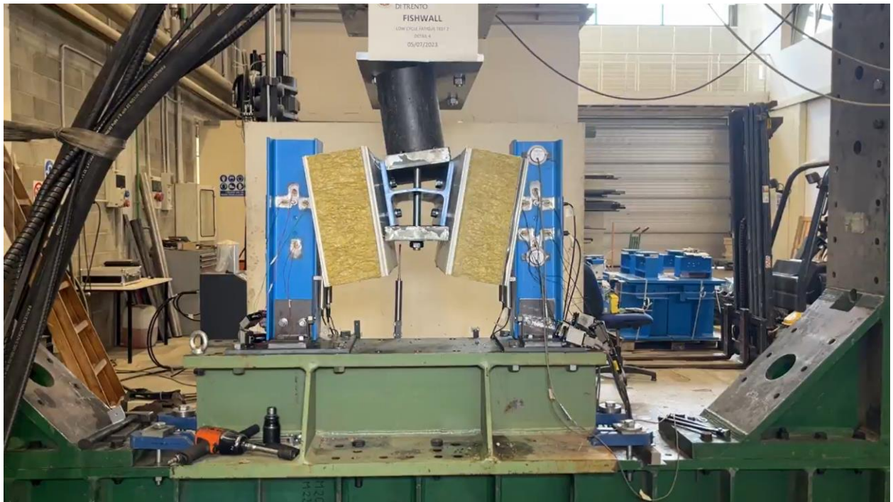
Figure A69. Detail 4 - cyclic test – deformation to +2\epsilon_y
