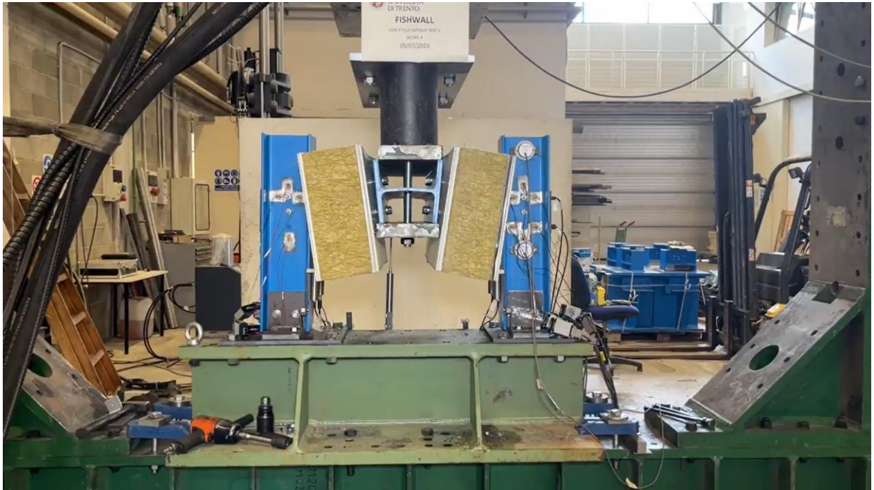
Figure A67. Detail 4 - cyclic test – deformation to +2\epsilon_y
