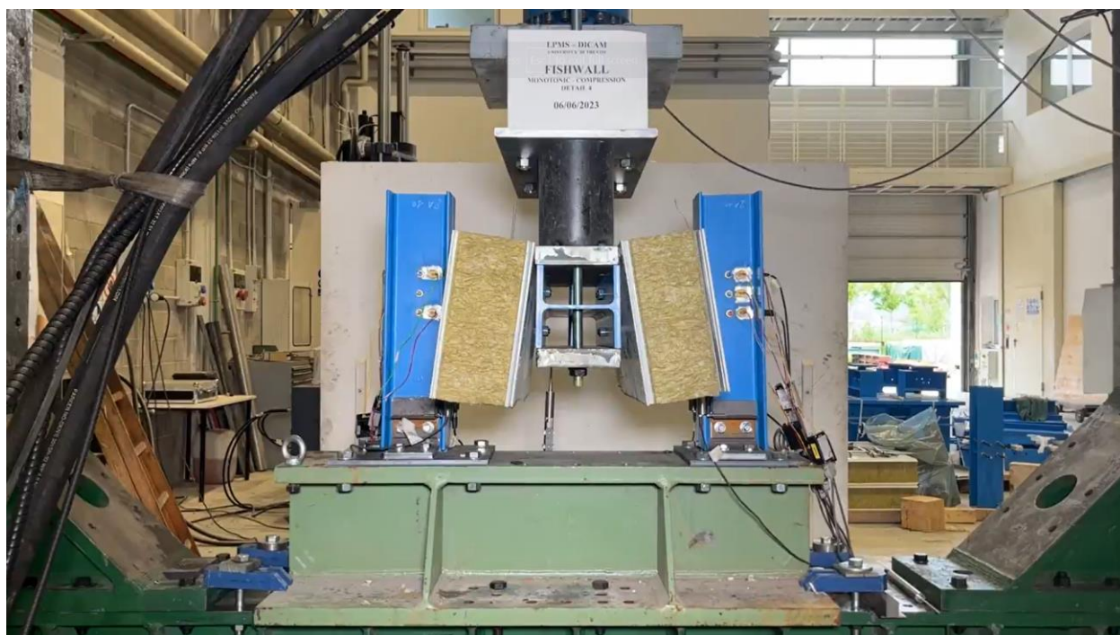
Figure A46. Detail 4 - compression test - deformation at 1.30 hour.
