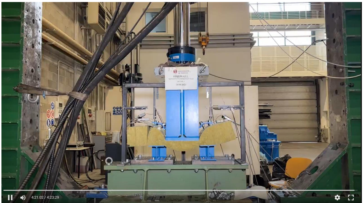
Figure A10. Detail 1 - compression test – deformation at failure
