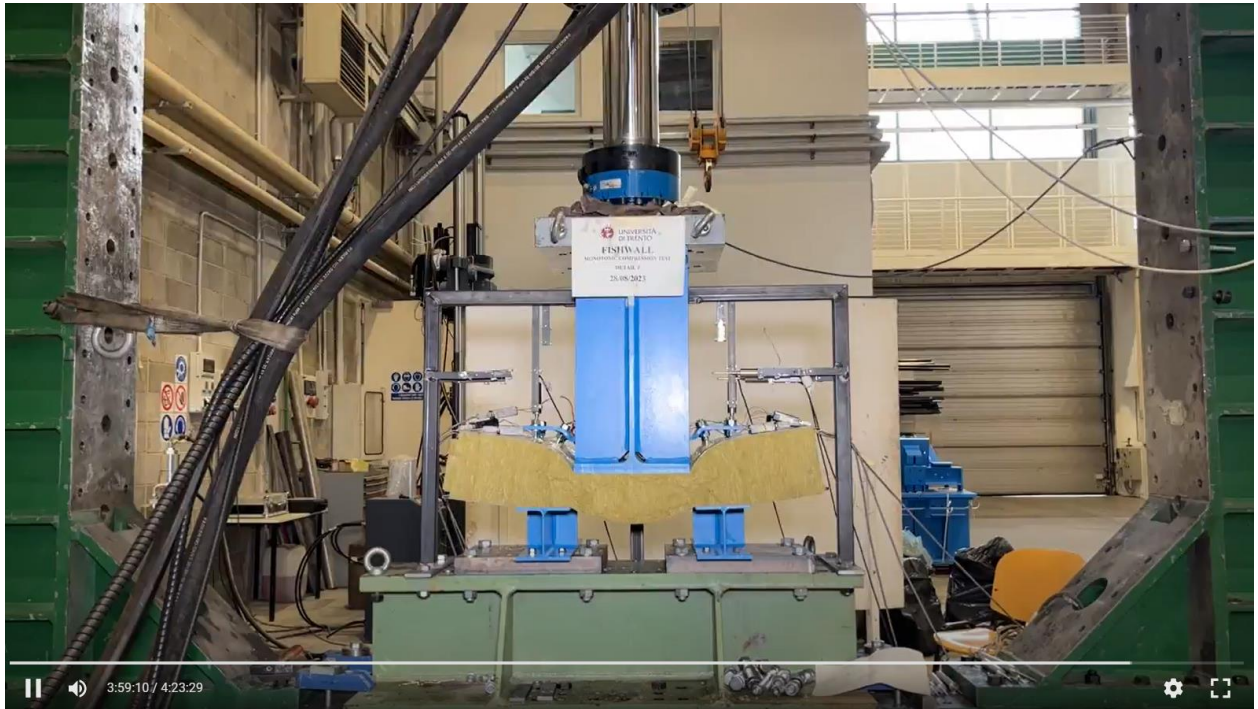
Figure A9. Detail 1 - compression test - deformation at 4 hours.
