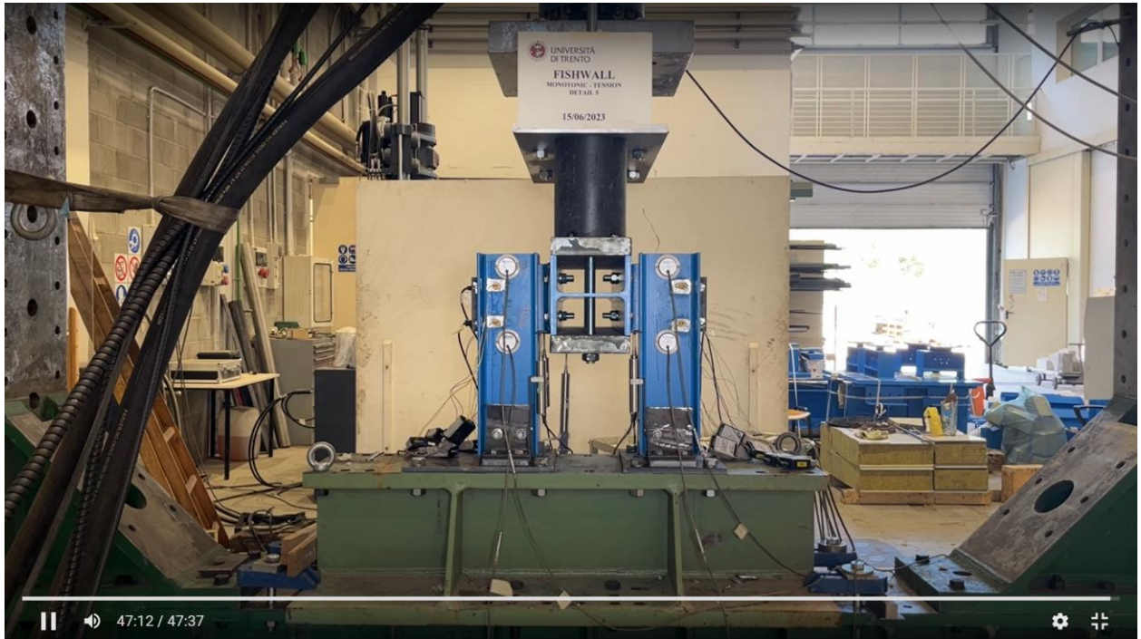
Figure A77. Detail 5 - tension test – deformation at failure.
