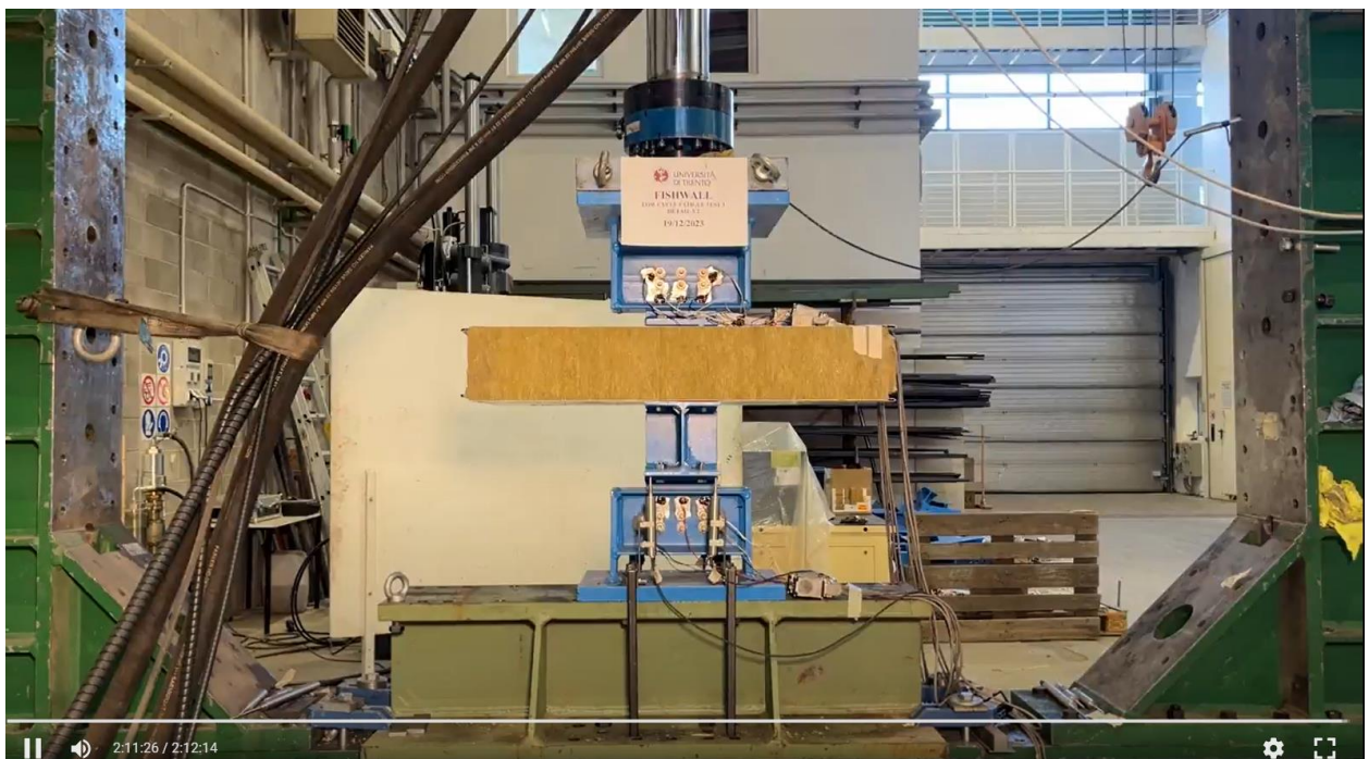
Figure A42. Detail 3.2 - cyclic test – deformation at failure.
