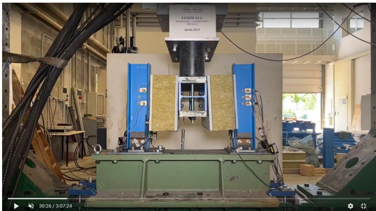
Figure A44. Detail 4 - compression test – deformation at 30 minutes.
