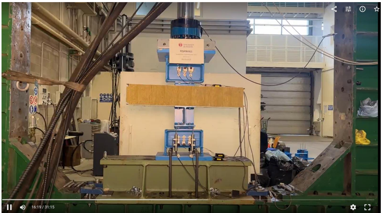
Figure A36. Detail 3.2 – compression test – deformation at 15 minutes.
