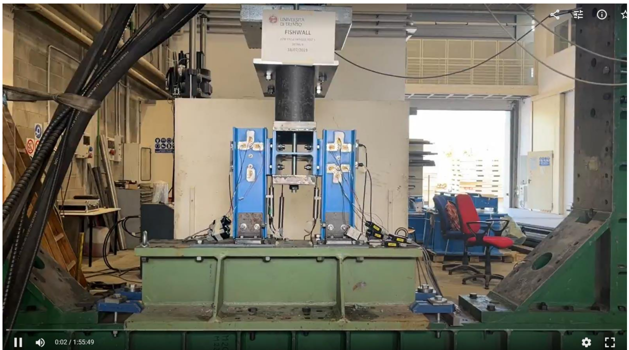
Figure A78. Detail 5 - cyclic test – beginning of the test.
