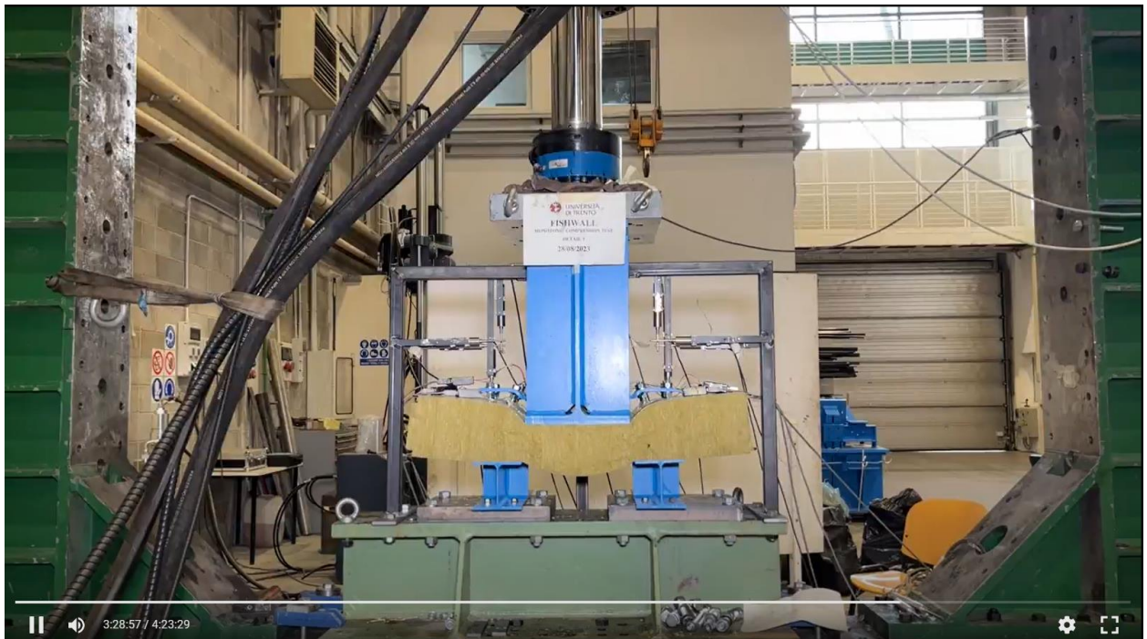
Figure A8. Detail 1 - compression test - deformation at 3.30 hours.
