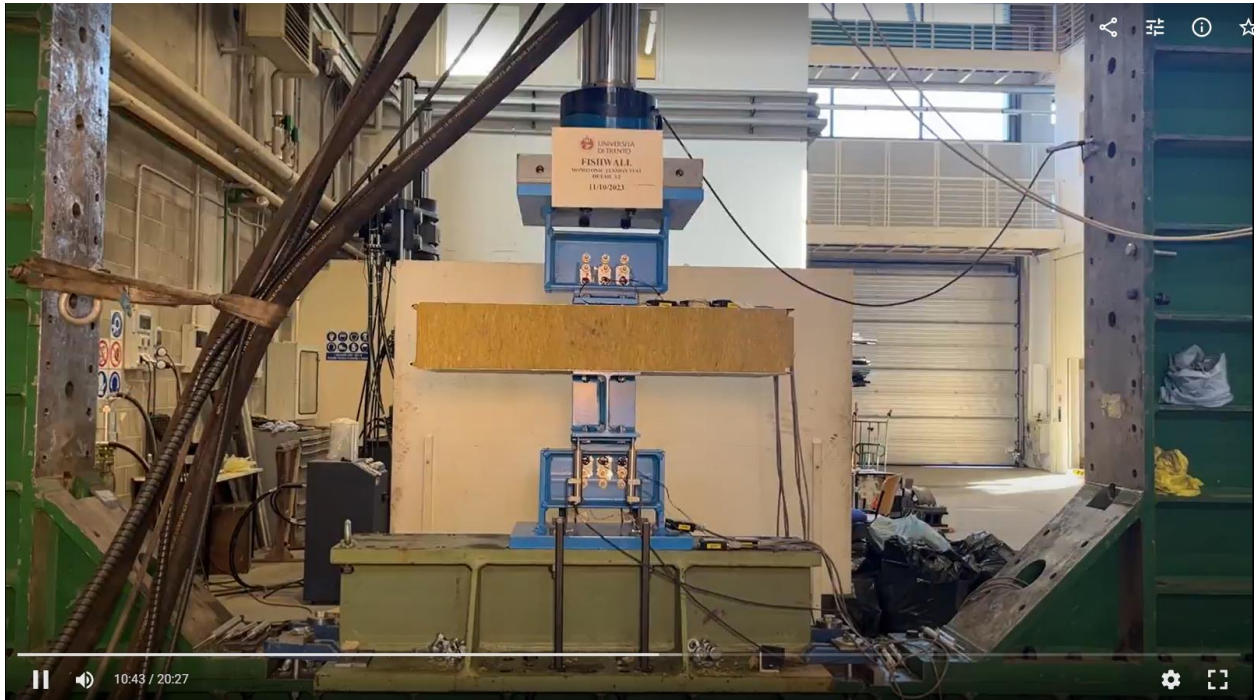
Figure A39. Detail 3.2 - tension test – deformation at 10 minutes.
