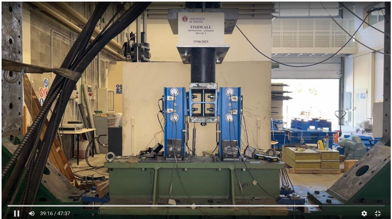
Figure A76. Detail 5 – tension test - deformation at 40 minutes.
