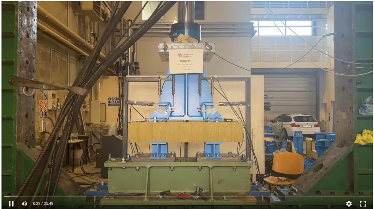
Figure A23. Detail 2 - tension test – beginning of the test.
