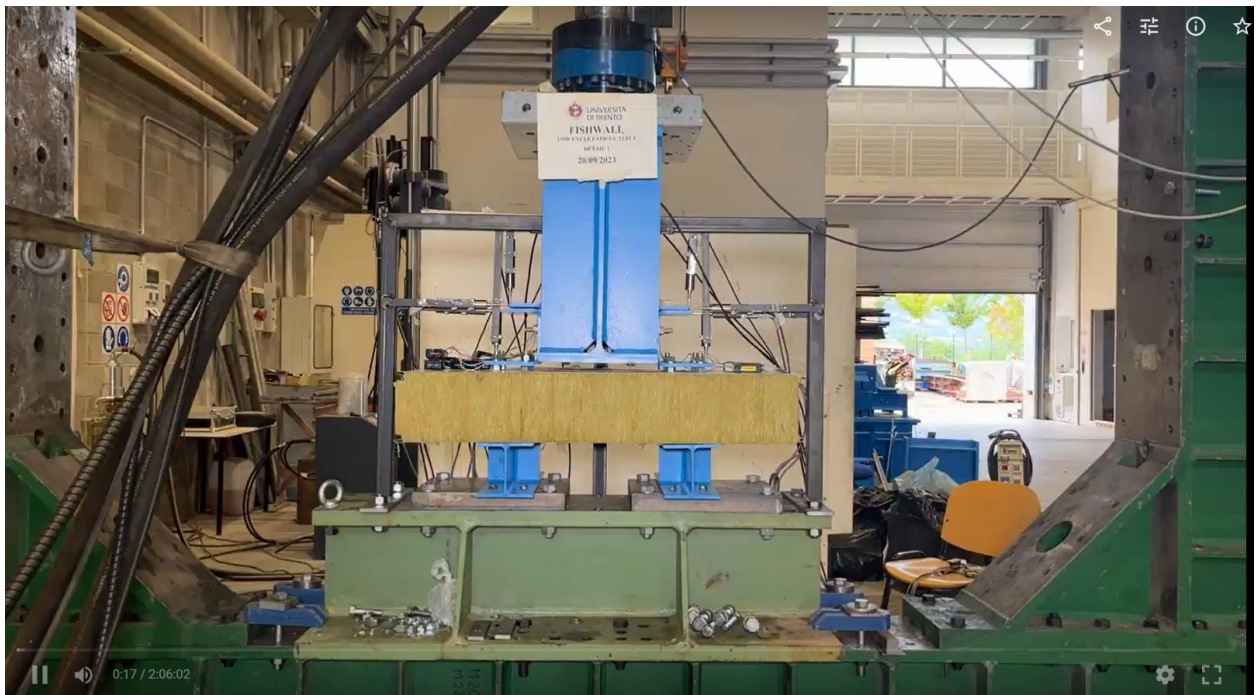
Figure A14. Detail 1 - cyclic test – beginning of the test.
