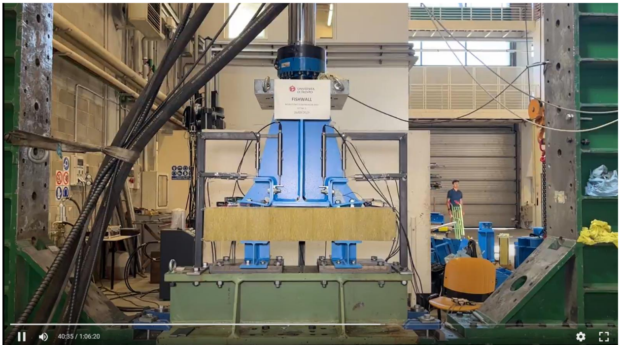
Figure A18. Detail 2 - compression test – deformation at 40 minutes.
