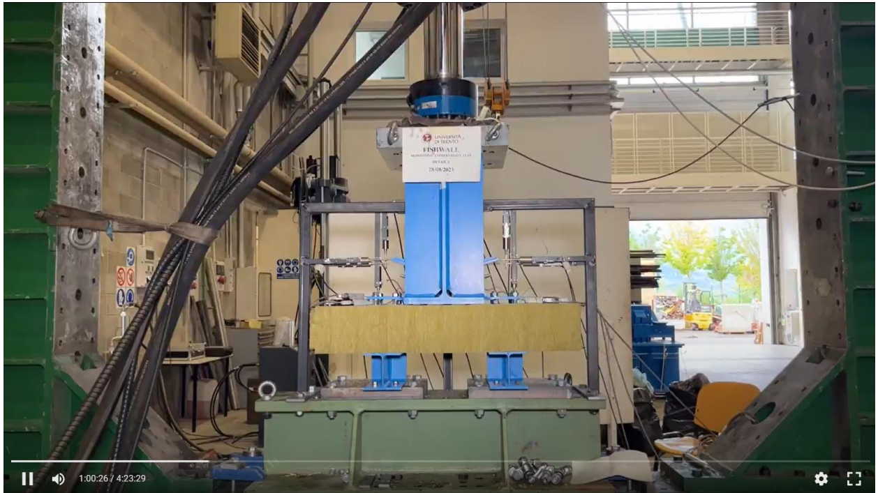
Figure A3. Detail 1 - compression test - deformation at 1 hour.
