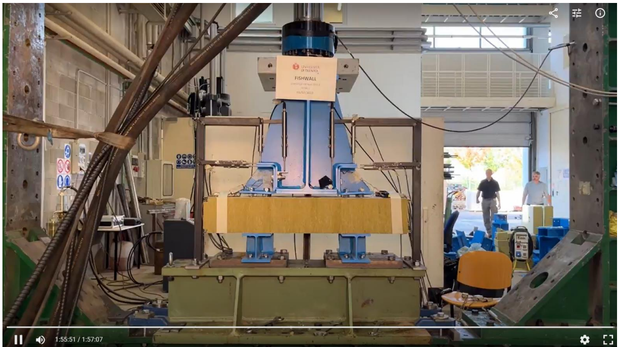
Figure A28. Detail 2 - cyclic test – deformation at failure.
