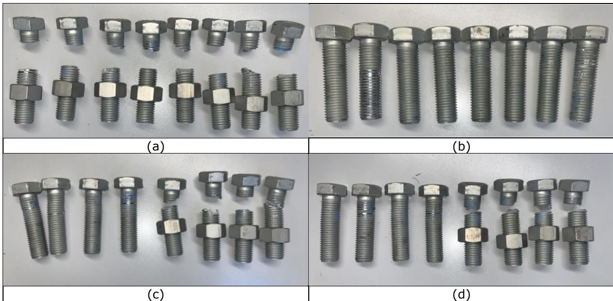
Figure 55. Detail 2 aluminium bolts at failure: (a) tension test; (b) compression test; (c) cyclic test 1; (d) cyclic test 2.
