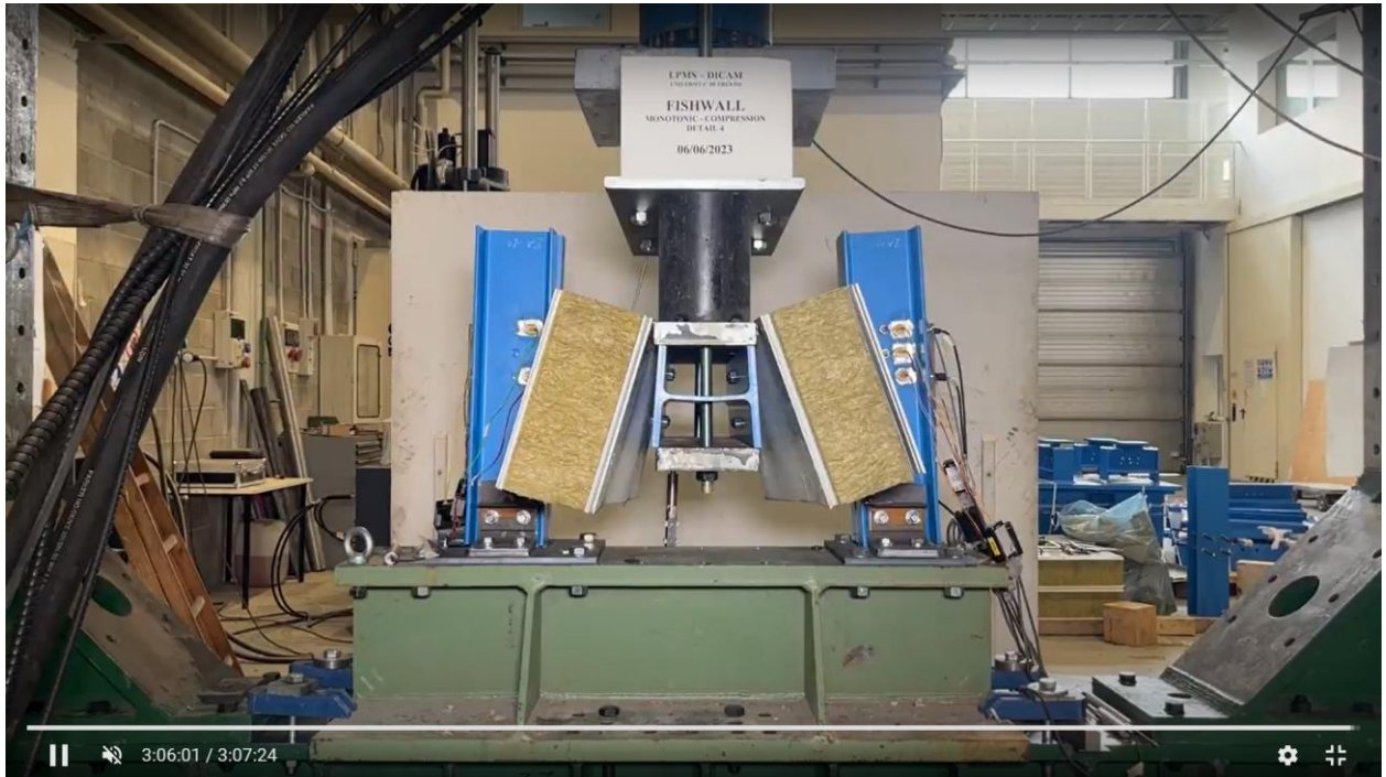
Figure A49. Detail 4 - compression test – deformation at failure
