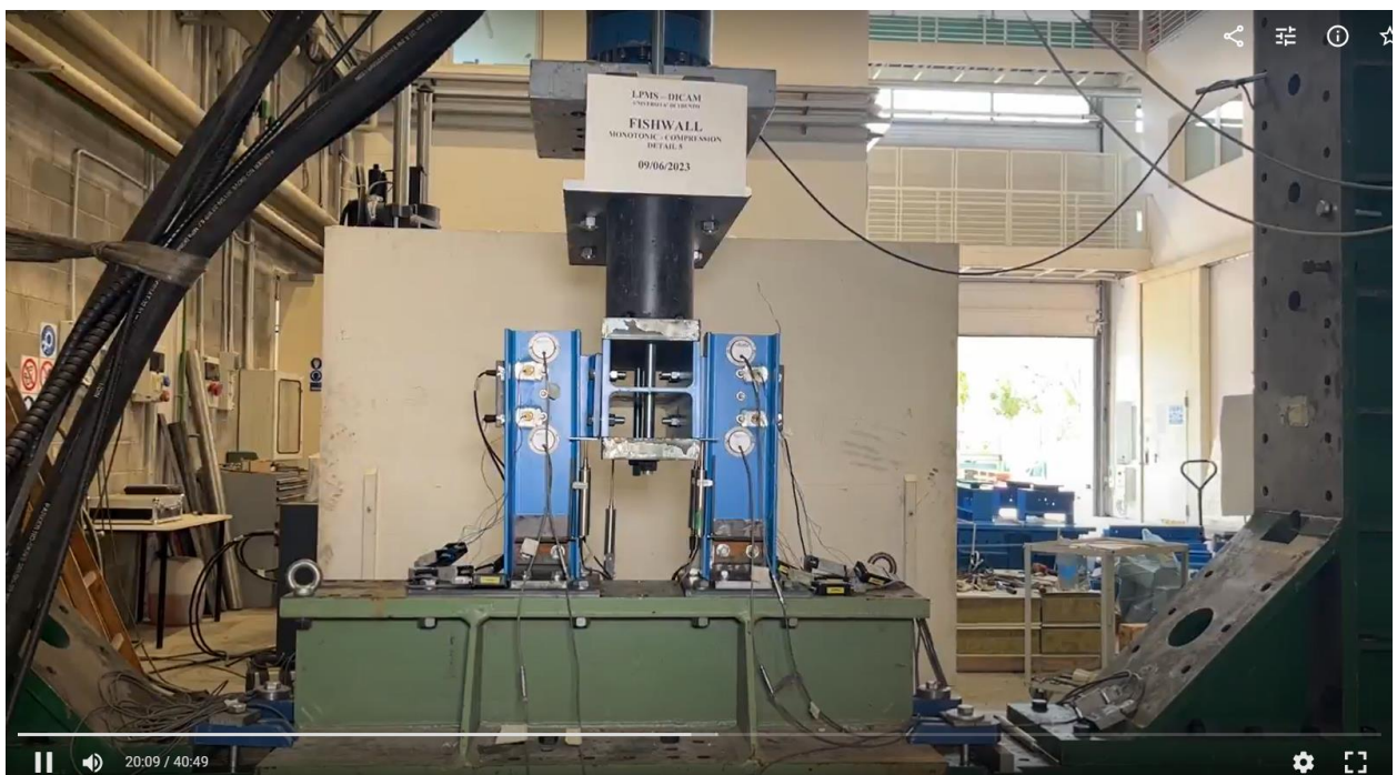
Figure A72. Detail 5 - compression test – deformation at 20 minutes.
