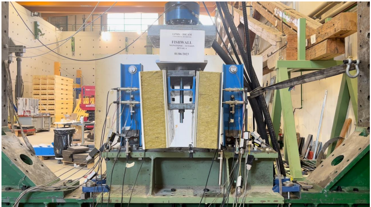
Figure A52. Detail 4 - tension test - deformation at 1 hour.
