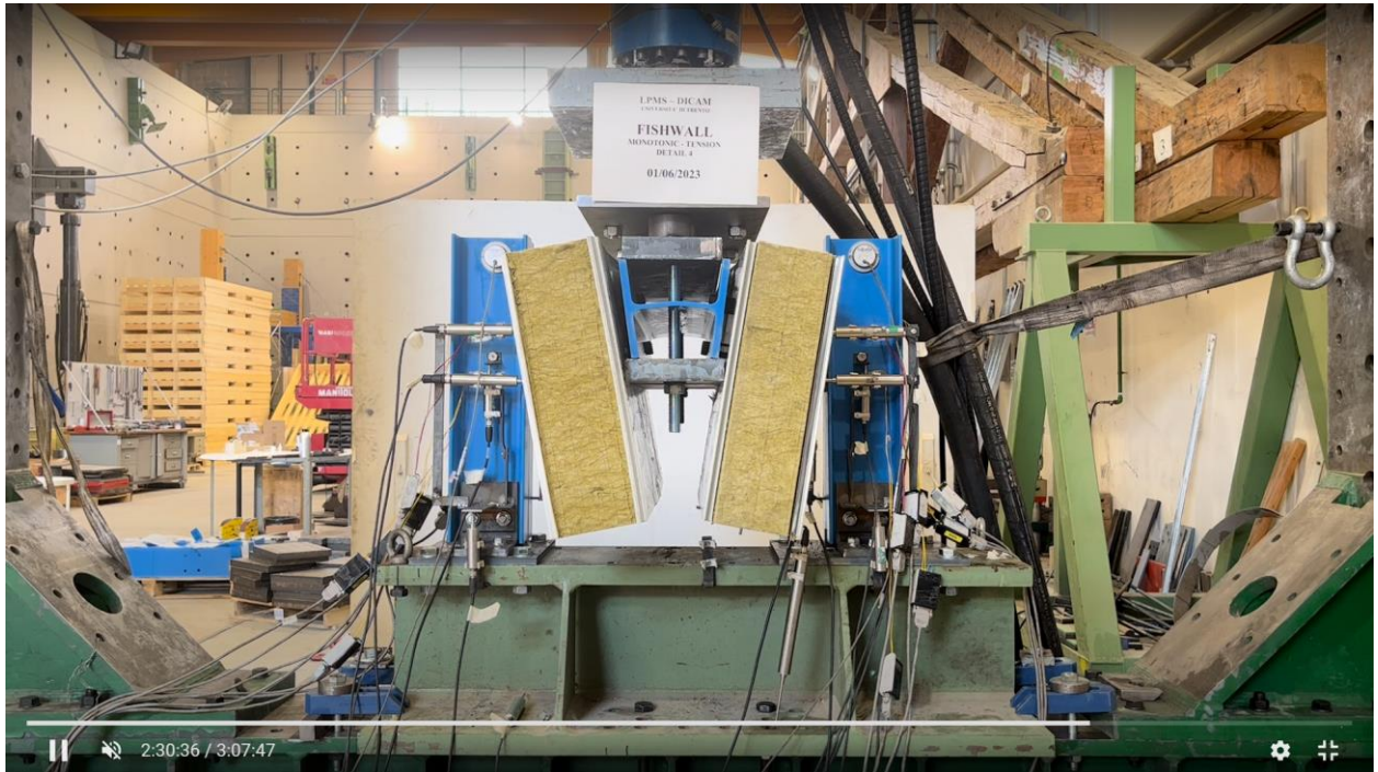
Figure A55. Detail 4 - tension test -deformation at 2.30 hours
