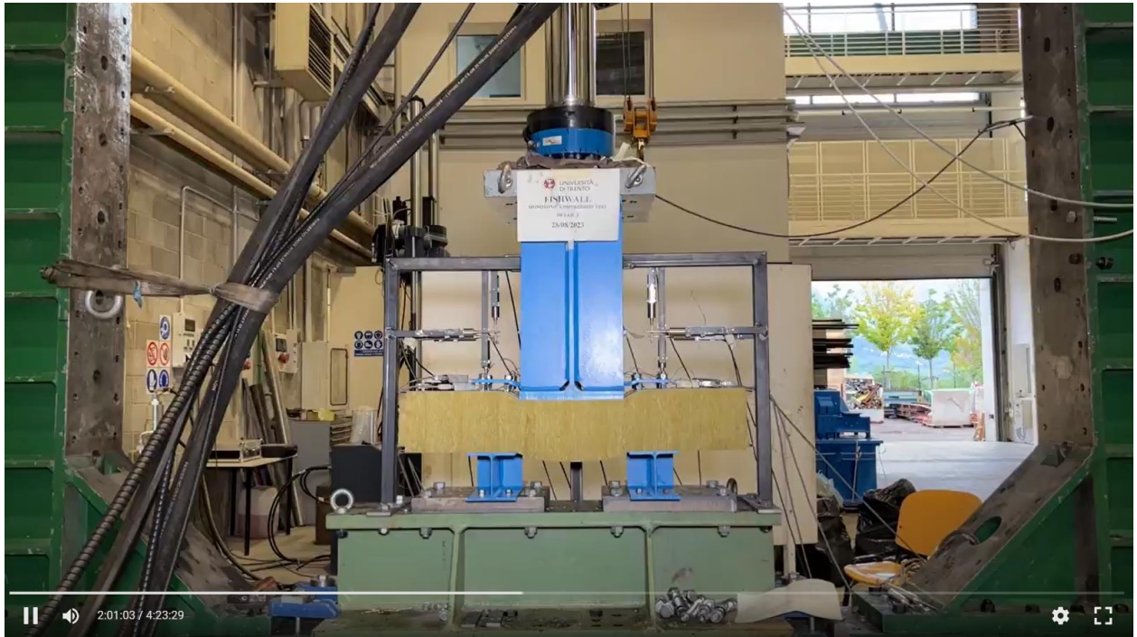
Figure A5. Detail 1 - compression test - deformation at 2 hours.
