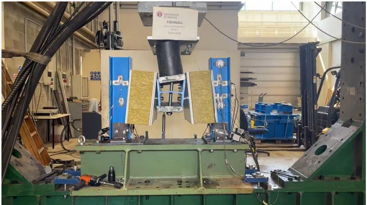
Figure A70. Detail 4 - cyclic test – deformation at failure
