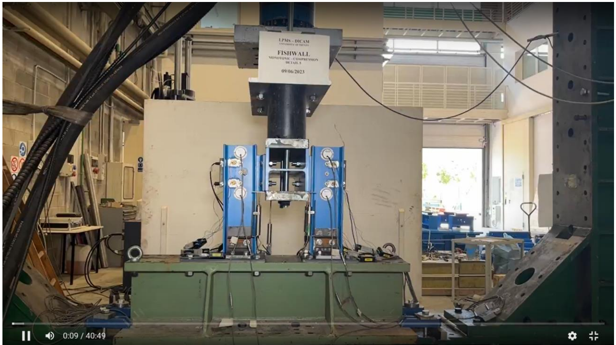
Figure A71. Detail 5 - compression test – beginning of the test.
