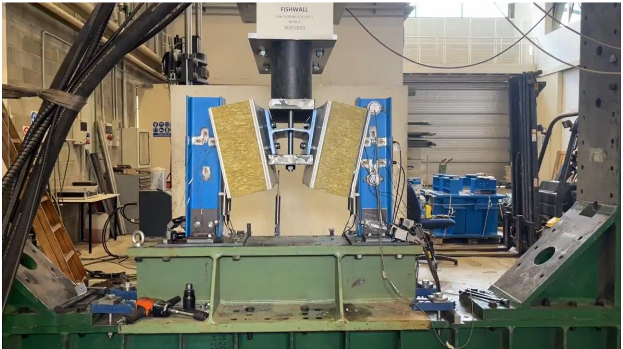
Figure A68. Detail 4 - cyclic test – deformation to +2\epsilon_y
