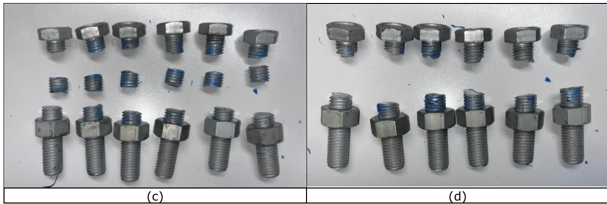
Figure 166. Detail 4 aluminium bolts at failure: (a) tension test; (b) compression test; (c) cyclic test 1; (d) cyclic test 2.
