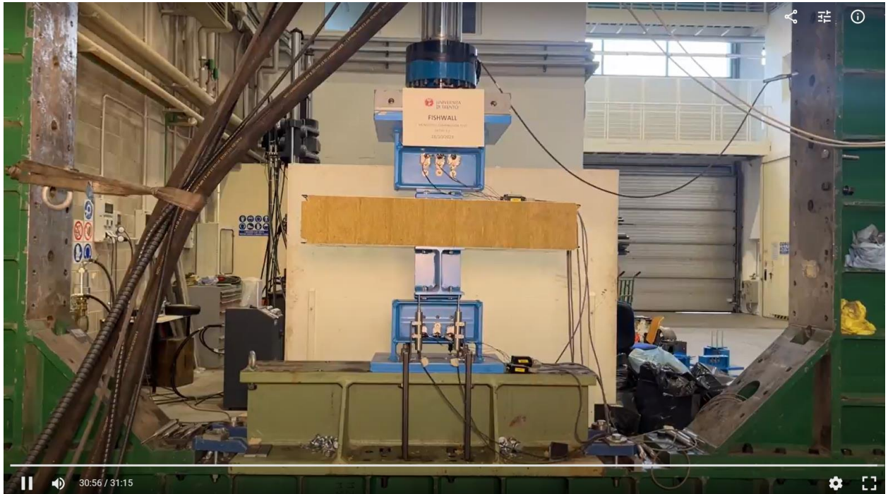
Figure A37. Detail 3.2 - compression test – deformation at failure.
