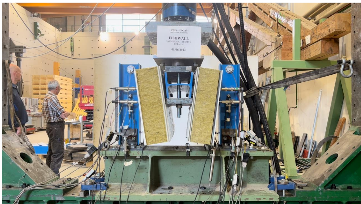
Figure A54. Detail 4 - tension test - deformation at 2 hours.
