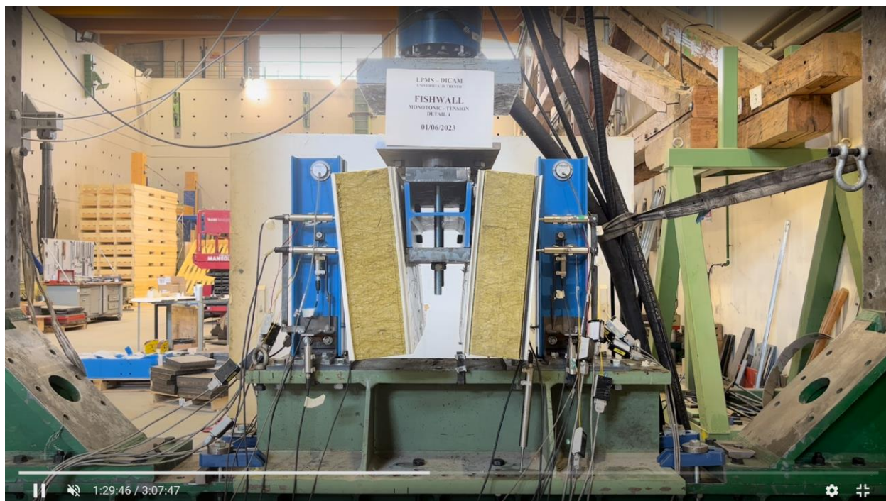
Figure A53. Detail 4 - tension test – deformation at 1.30 hour
