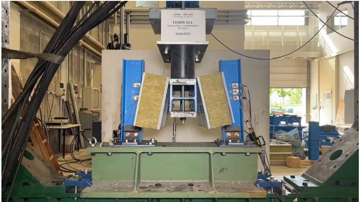
Figure A47. Detail 4 - compression test - deformation at 2 hours
