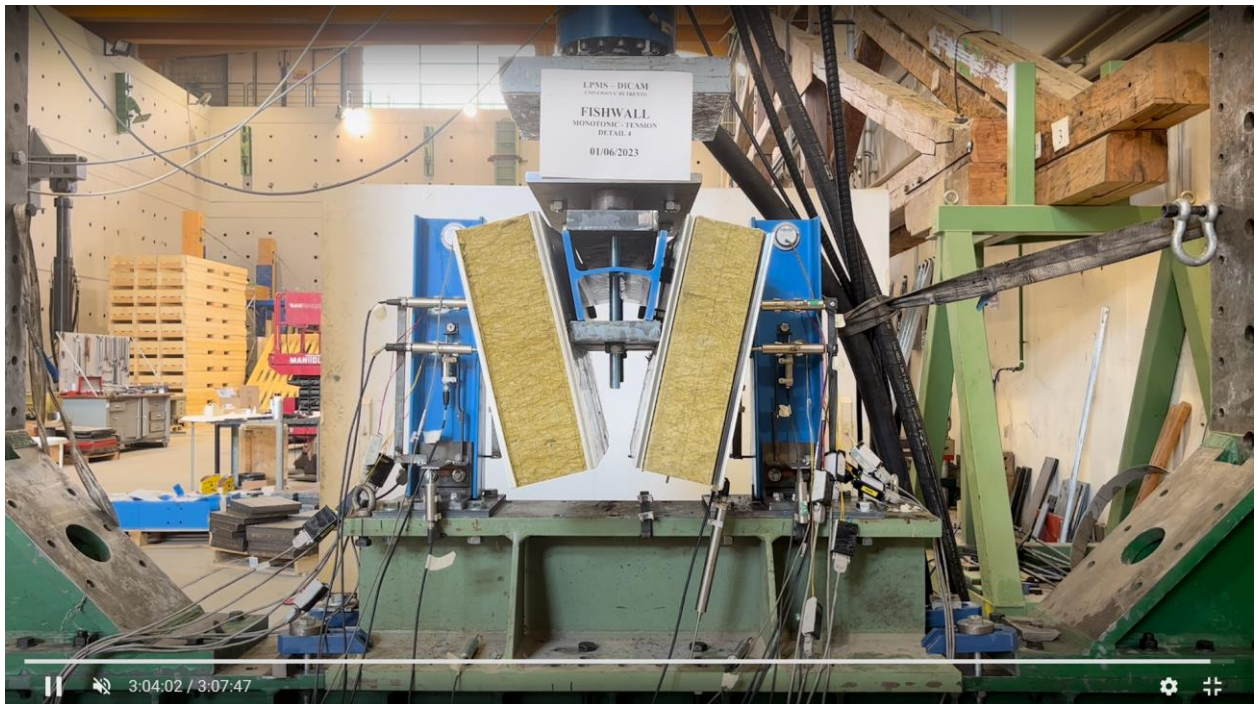
Figure A56. Detail 4 - tension test - deformation at 3 hours.
