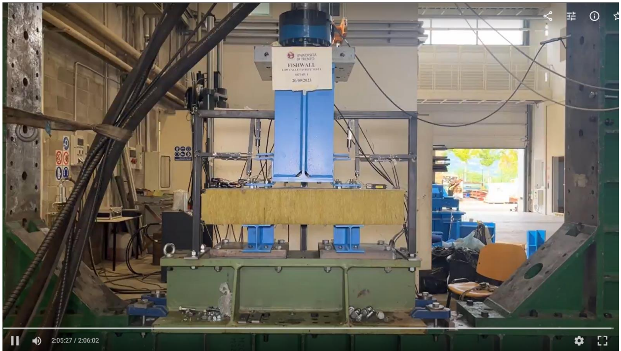
Figure A15. Detail 1 - cyclic test – deformation at failure
