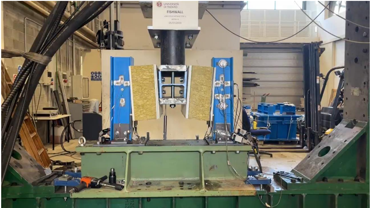
Figure A65. Detail 4 - cyclic test – deformation at e_y
