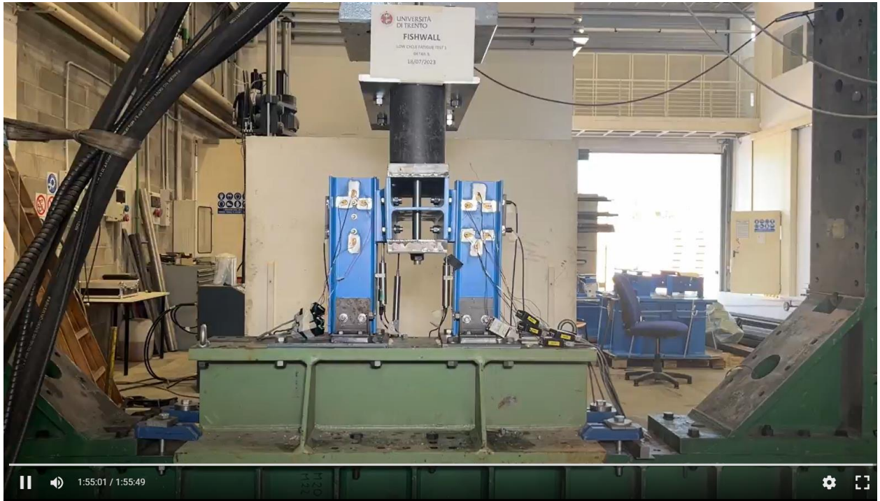
Figure A79. Detail 5 - cyclic test – deformation at failure.
