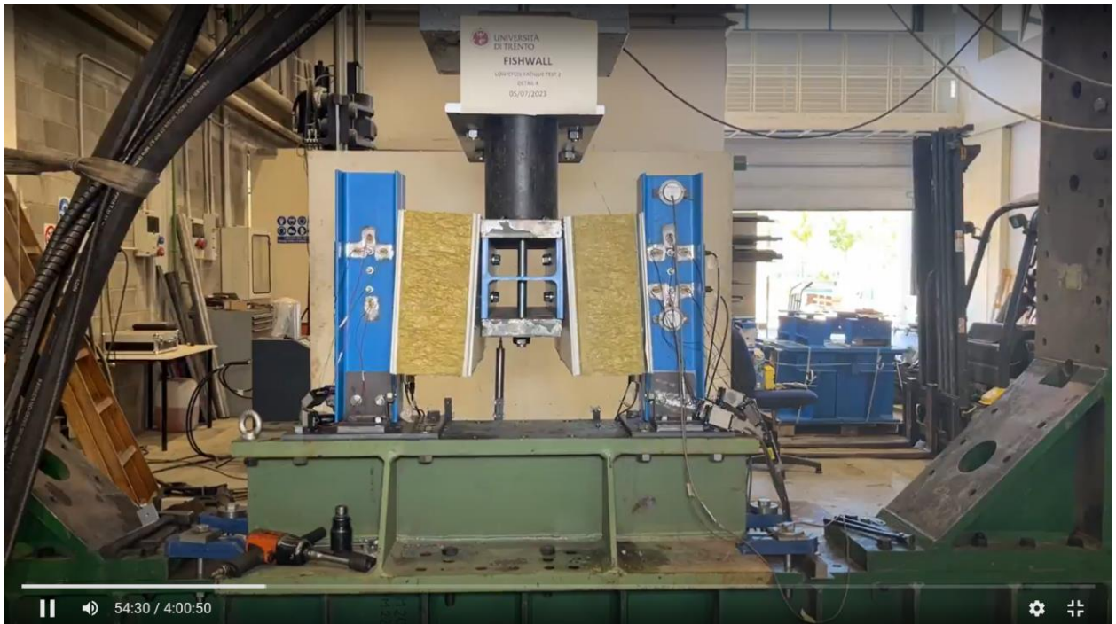
Figure A62. Detail 4 - cyclic test – deformation at -e_y/3
