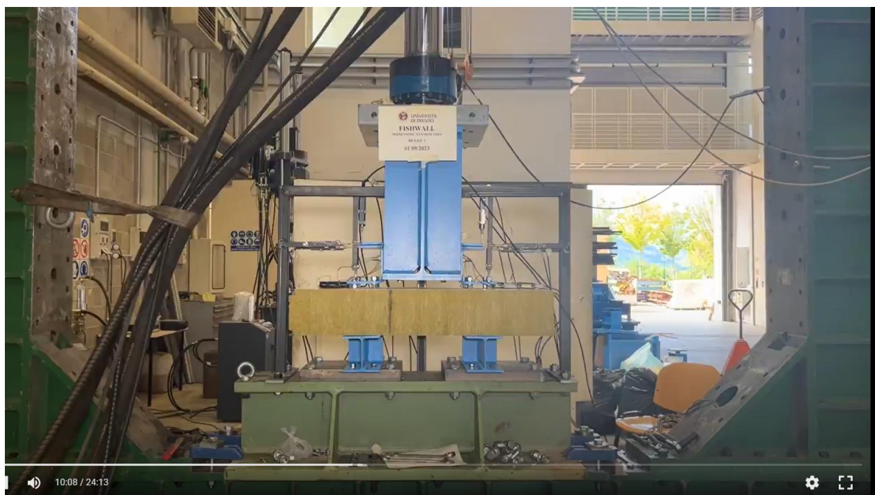
Figure A12. Detail 1 - tension test – deformation at 10 minutes.
