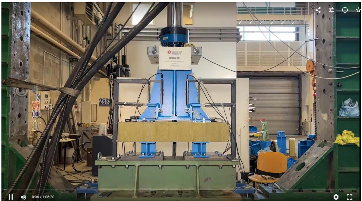
Figure A16. Detail 2 - compression test – beginning of the test.
