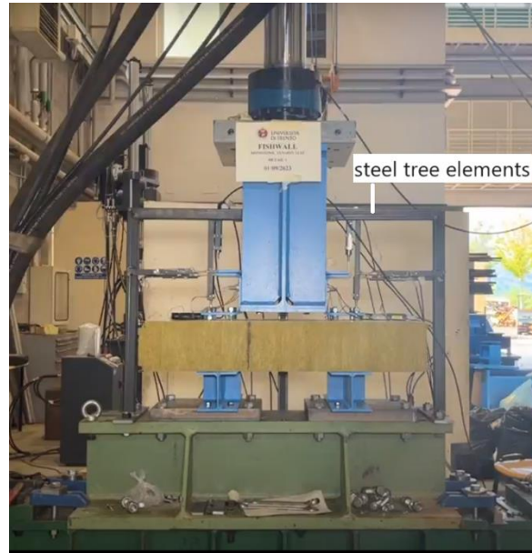
Figure 6. View of the tension test set-up for detail 1.
