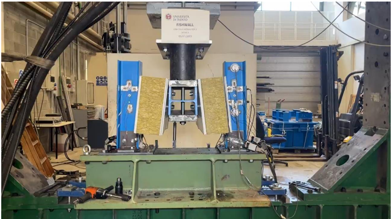
Figure A66. Detail 4 - cyclic test – deformation at -e_y
