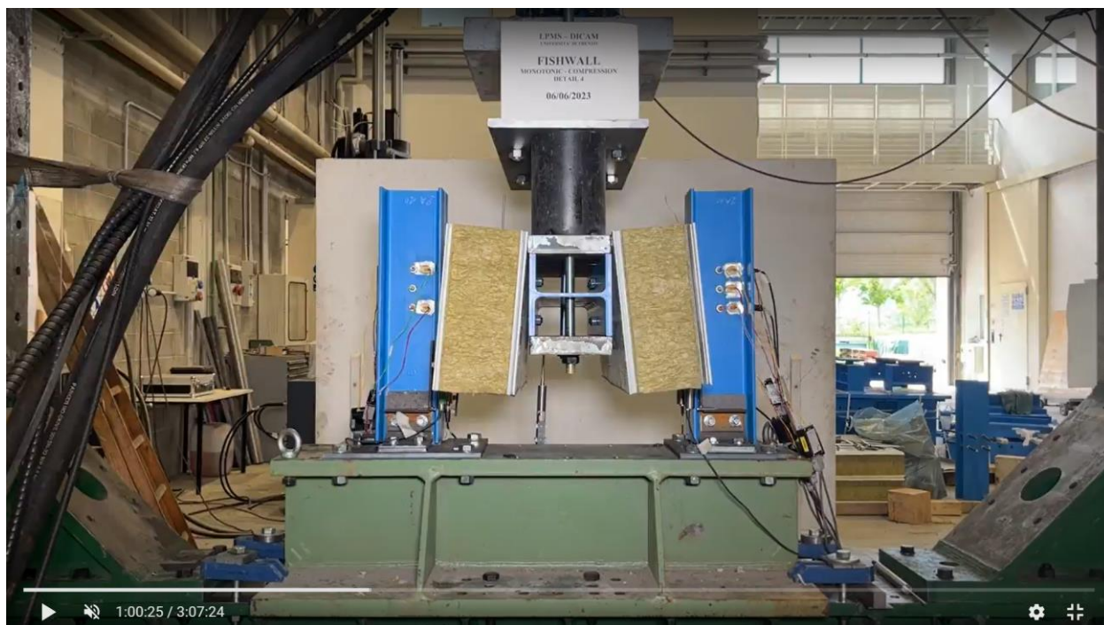
Figure A45. Detail 4 - compression test - deformation at 1 hour.
