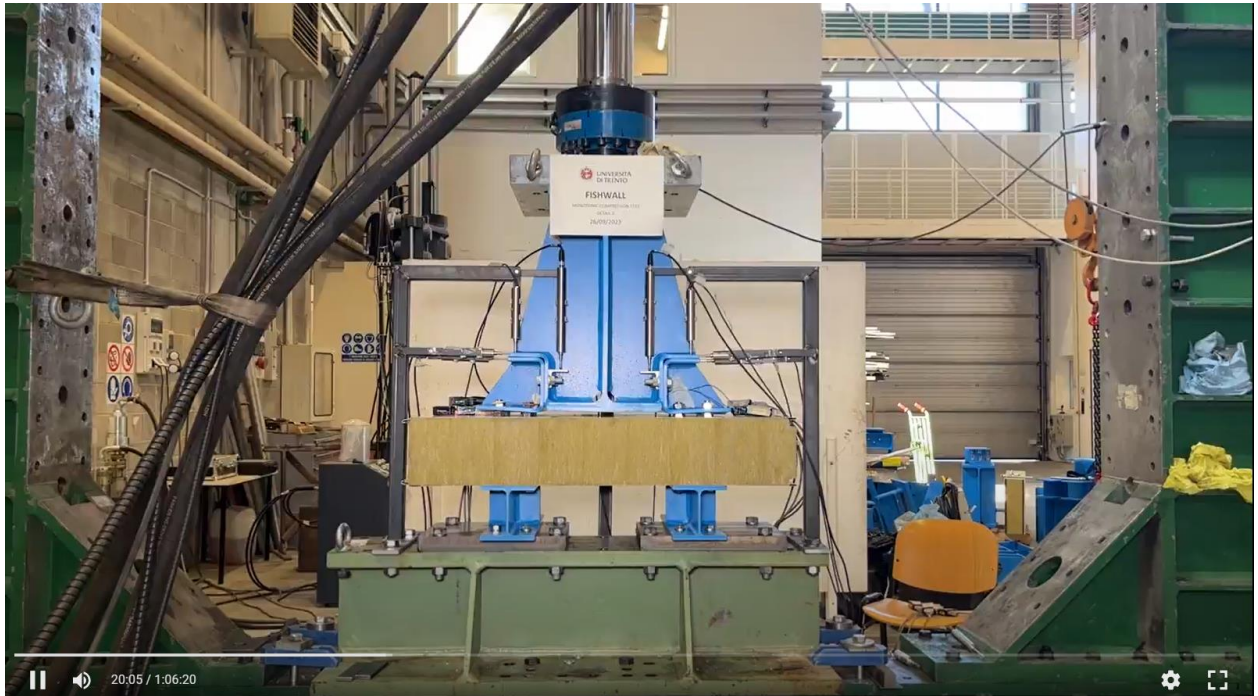
Figure A17. Detail 2 - compression test – deformation at 20 minutes.
